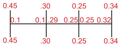
Figure 4.5.4: distribution factors along E2-F4-F7 on level 2
