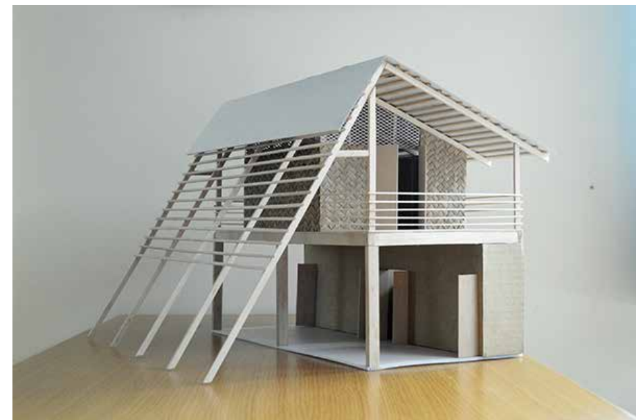
7. Scaled model for a low cost housing unit for Habitat for Humanity. The use of model makes communication easier between project stakeholders.
